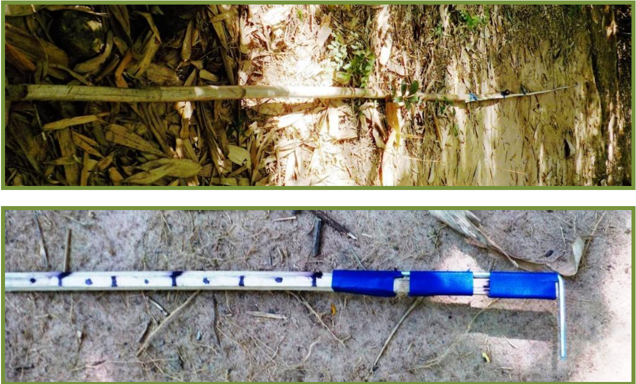
Figure 6. The split bamboo pole (top) used for measuring tall culm shoots, and the bracket at its apex (bottom).
