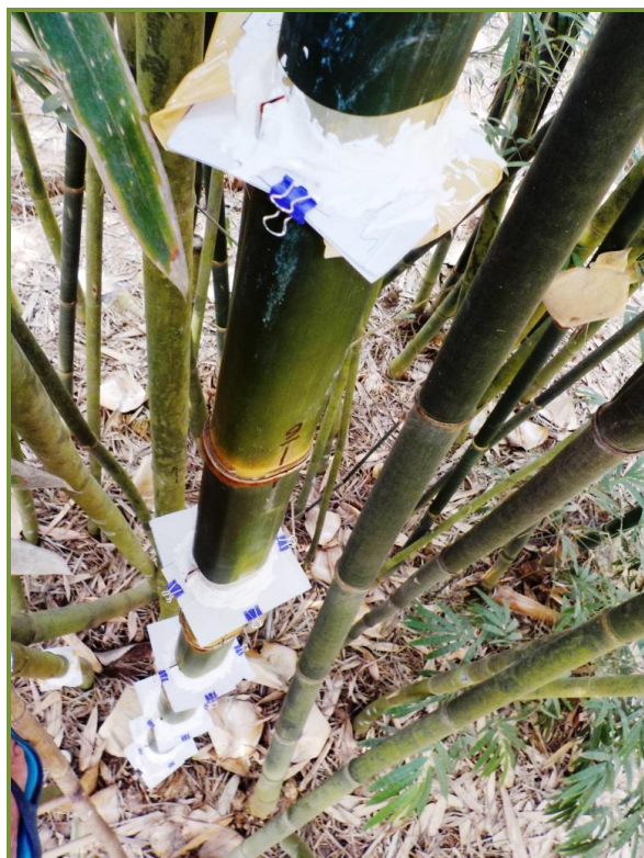
Figure 18. The trained culm clearly showing a modified, and tending square, XS. In the photo the XS forms are clipped and plastered in place.
