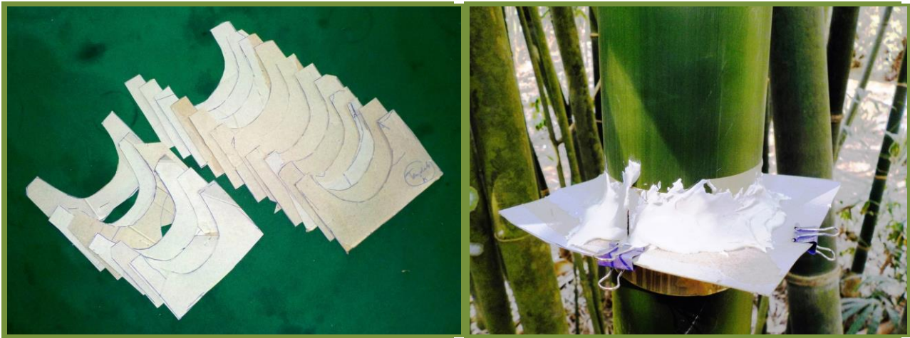
Figure 7. Cardboard cut-outs to make XS profiles (left), and clipped and plastered in place on the trial culm (right). One pair of flanges can just be seen next to the clip on the left.
